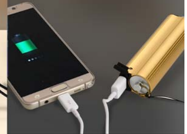
Emergency Power Bank
